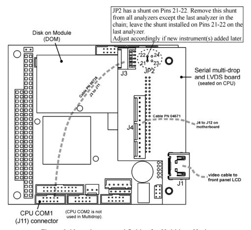
Figure 3-16: Jumper and Cables for Multidrop Mode
